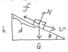
$$\begin{split} E_{k,i} &= 0, \quad U_i = mgh = mgd\sin\theta \\ T_f &=? \quad U_f = 0 \quad \Rightarrow T_f = mgd\sin\theta - mgd\cos\theta\mu = \frac{1}{2}mv_f^2 \\ v_f &= \sqrt{2gd(\sin\theta - \mu\cos\theta)} \end{split}$$
